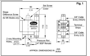
These pressure switches can be mounted in any direction.
