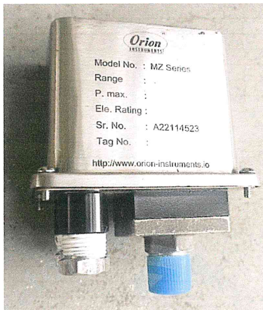
Picture1: Pressure Switch
