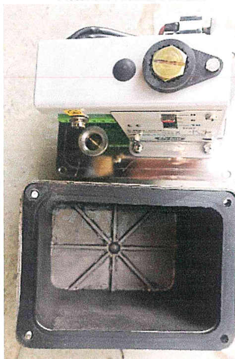
Picture2: No ingress of powder & water observed
